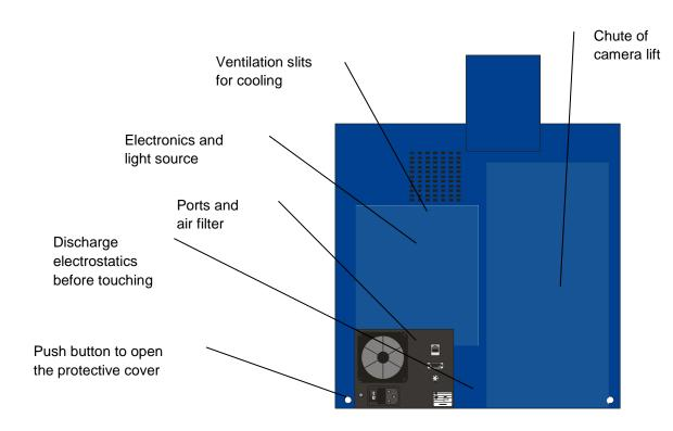
The ventilation slits of the cooler must always be open!
