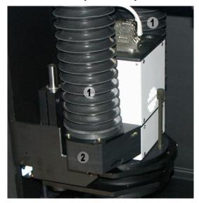
era using a cable holder. The filter block of the power supply cable is fixed to the top of the camera using Velcro fastener.
