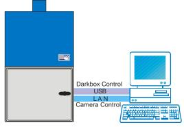
An Ethernet as well as an USB-connection connection is required to control the NightOWL II with NC100e or NC320e camera and to transfer data. An additional network adapter (PCI card, USB) is needed to connect the PC to the local network (Internet access, network printer, etc.)
