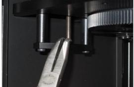
Turn the shaft until the focus drive moved down approx. 5 mm.
