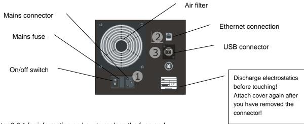
see chapter 8.2.1 for information on how to replace the fuse and how to clean the air filter.
