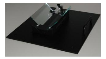
The Mirror assembly is located on a special carrier. This carrier is placed on a base plate which is positioning the carrier under the camera. On the carriere there is a single anaesthesia mask to anesthesise the animal during the maeasurement..
