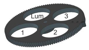
Please observe the correct installation direction (arrow on the filter wheel) when loading the filter. Please refer to the filter manufacturer's description. The filters should be secured from above against falling out by the snap rings which are included with the device. For installation, slide the filter wheel onto the shaft until you feel distinctly that is has snapped into place. Then click introduced from the Acquisition dialog box (Start an Acquisi-
