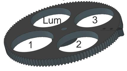
The positions of the filters are numbered and identified by a respective number printed on the filter wheel.
