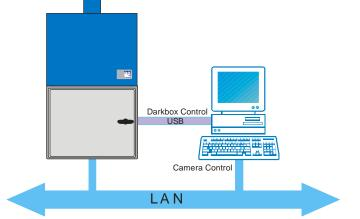
If the NightOWL II is connected via local network installation (wall outlets or network switch), you must observe the local IP address range to rule out possible double assignment of IP addresses of the NightOWL II.
