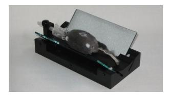
As sample format select a sample size of 130mm. The sample height should be set to 25mm plus the half of the height of the measured animal. This means with an animal height of 20mm a sample height of 35mm.
