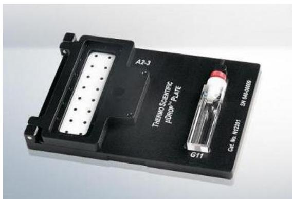
**Figure 1:** The  $\mu$ Drop plate can be used for DNA quantification using absorbance in a microplate reader using only 2  $\mu$ L of sample and also features a cuvette port for increased flexibility.
