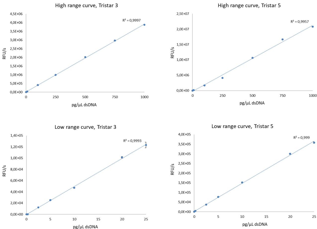
**Figure 2:** dsDNA standard curves measured with a Tristar 3 (left) and Tristar 5 (right) Multimode Reader with standard fluorescein filters. All measurements in triplicate. Data are average  $\pm$  SEM.
