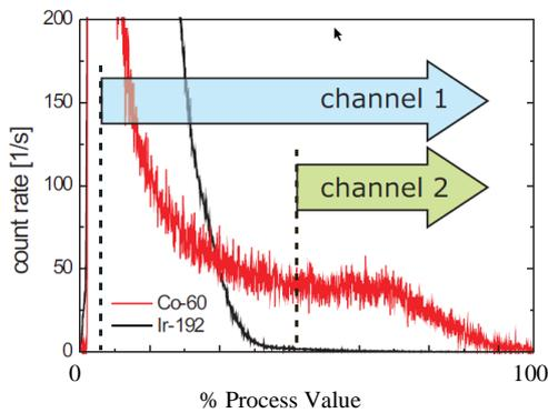
every recognized gamma particle is counted. Another channel (Channel 2) covers the higher energetic pulses only. Thus, lower energy pulses i.e. from weld inspection sources, which do not exceed a certain height are therefore not recorded in channel 2. All pulses above the threshold for Channel are exclusively from the C-60 source of the measurement system.
