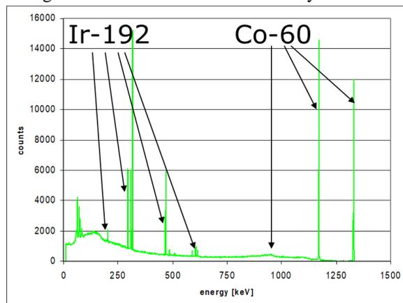
In theory Iridium - 192 and Cobalt - 60 have their distinct energy and an energy spectrum looks like the above picture. In reality, not every gamma particle deposits his complete energy in the scintillator. Depending how the gamma quant hits the scintillator it leaves without having transformed the full amount of energy. Thus, a real energy spectrum looks like the following graph:
