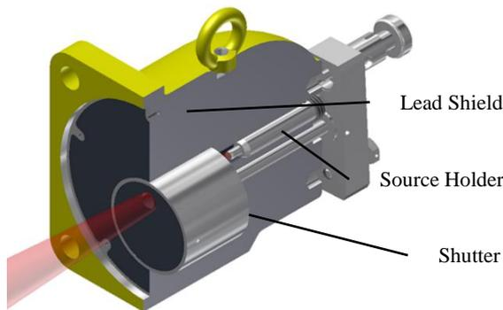
Fig. 2. Source container (shield) of a point source
