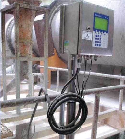
In the Sugar Production process, concentration measurement and control of milk of lime is critical to insure proper quality and cost stability.
