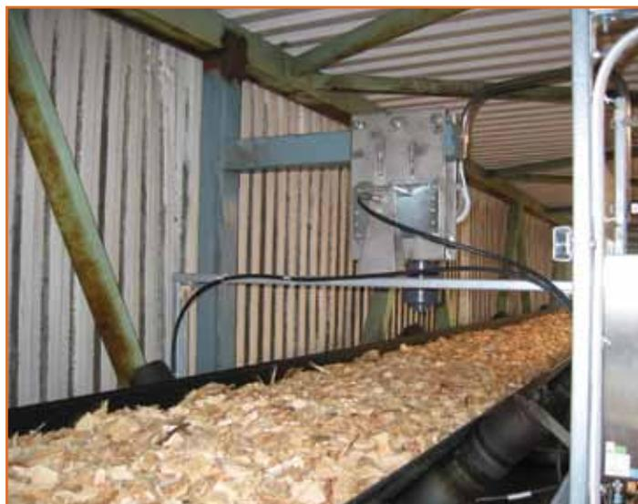
MicroPolar moisture analyser from Berthold Technologies installed on a woodchip conveyor (with bulk density compensation)
