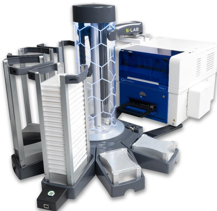
The S-Lab™ Pro automated plate handler attached to the Tristar 5 Multimode Reader
