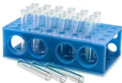
We offer sample tubes for luminescence detection in different heights/volumes, which are suitable for measurements in tube luminometers. The tubes are made of polystyrene, have a diameter of 12 mm and fit all our tube luminometers.
