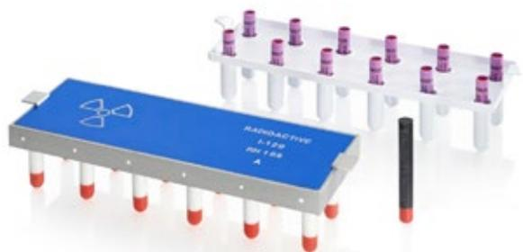
Our gamma test sources are designed to facilitate your QC and QM . We provide single-tube or 12-tube  $^{129}\text{I}$  or  $^{57}\text{Co}$  sources of 2 KBq/tube to help you calibrate and check the performance of your multi-well gamma counter.
