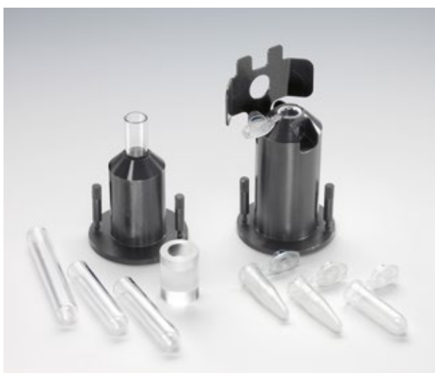
Figure 2: Unmatched sample format flexibility – from microcentrifuge tubes to standard luminescence tubes (picture includes optional accessories).
