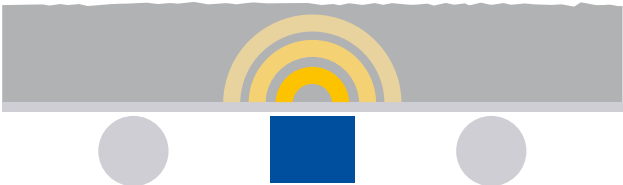
Schematic representation of neutron moisture measurement at a conveyor belt
