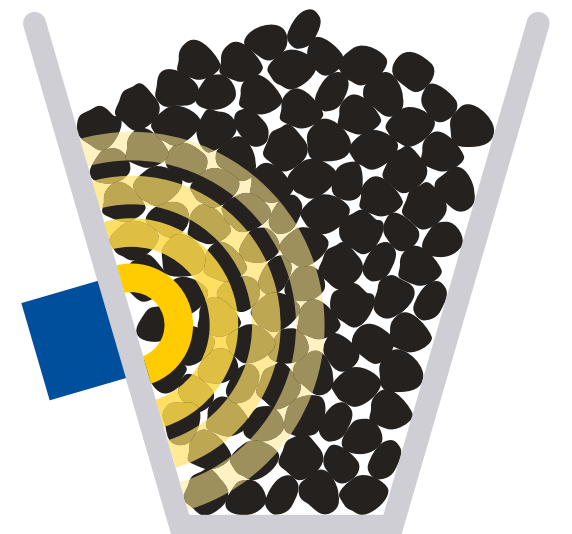
Schematic representation of neutron moisture measurement in vessel
