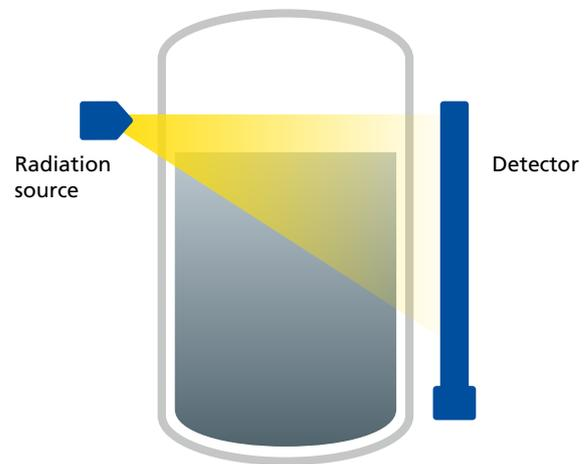
Fig. 2 Typical setup of a scintillation detector used for radiometry. The three main components
