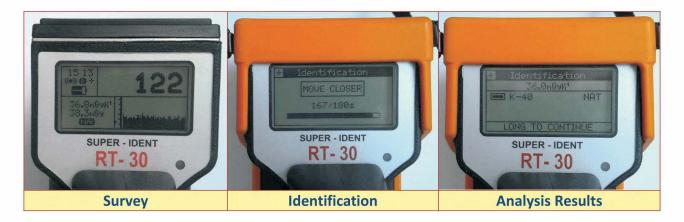
The RT-30 uses an advanced method of Automatic Stabilisation on Natural Background Radiation throughout its operation. This unique method eliminates the need for an additional radioactive check source.
