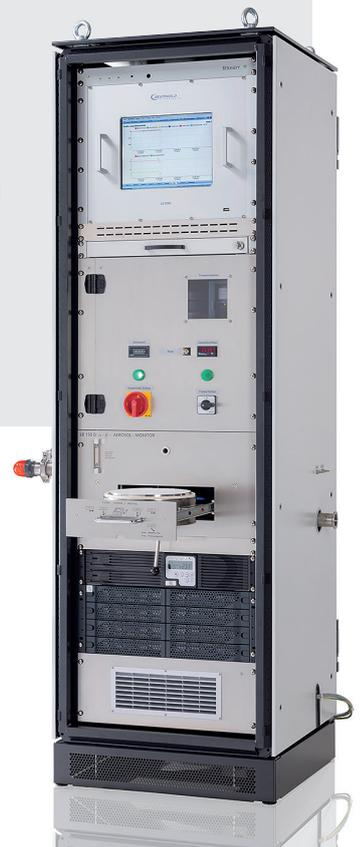
Figure 1: LB 150 D-R Alpha-Beta Fixed Filter Monitor with opened drawer of the particulates collection unit.
