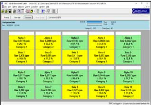
LB 790 AMS display of measurement values for all 10 detectors and both channels
