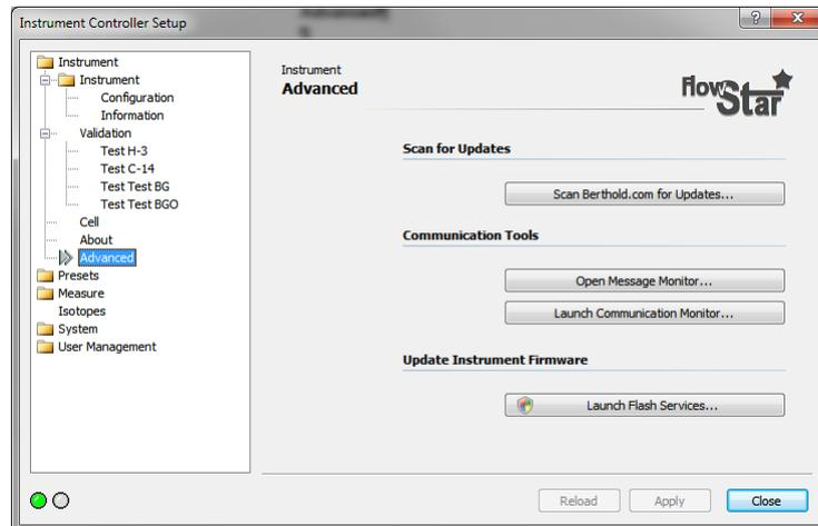
Advanced tools for software updates and monitoring are offered in this section. By clicking  the controller connects with the Berthold Technologies webpage and checks if a newer version of the controller is available and downloads it after confirming.
