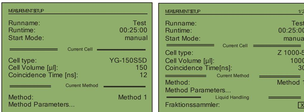
Figure 29: Liquid handling disabled (left) and enabled (right)
