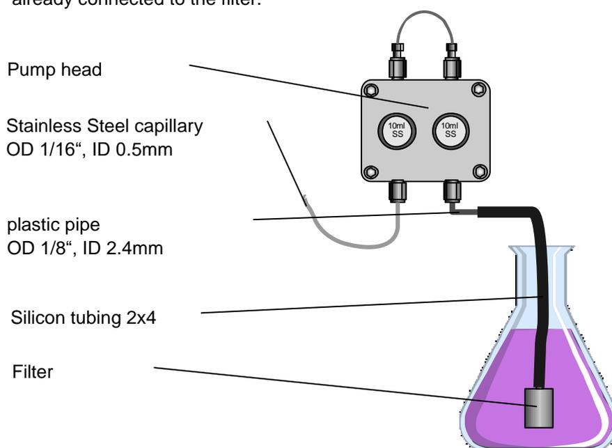
*The filter should always be clean.* In case of possible gel-like deposits or impurities, clean it using methanol or ethanol. For cleaning, the filter may be dismantled and the filter disc removed and, if necessary, replaced. The pump inlet fitting of the tubing is mounted as shown in the picture below.
