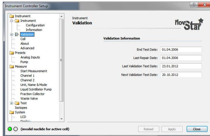
The “Validation” tab shows the dates of the validation process as well as upcoming test dates. In the subcategories Test H-3; Test C-14; Test BG; Test BGO the test results of the validation measurements as well as the first validation can be reviewed as a table or graph.
