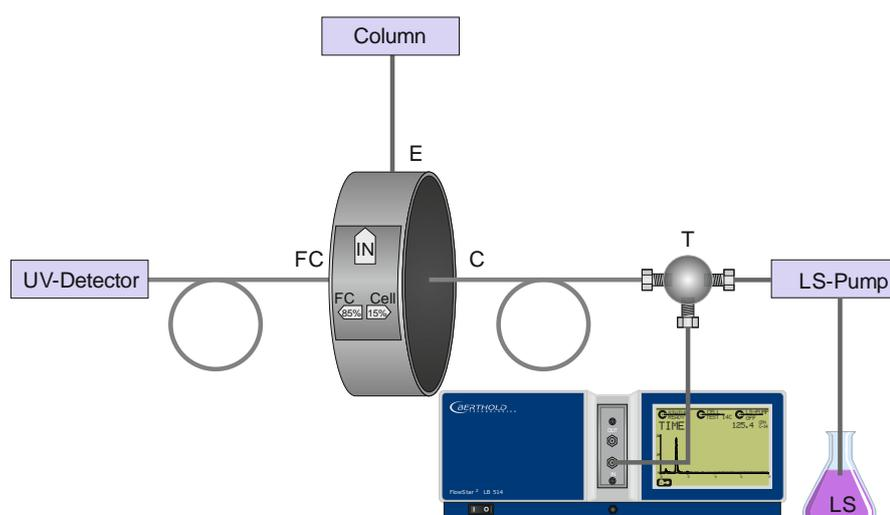
Figure 12: Configuration with subsequently connected UV detector
