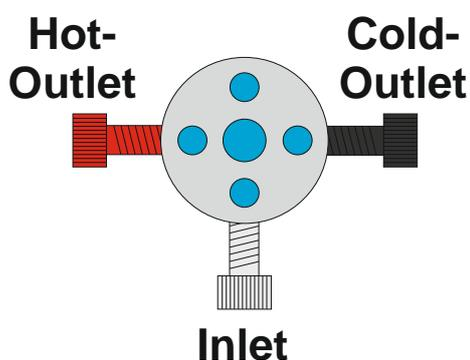
The outlet with the black color label is the so called “cold outlet”. This outlet is active if the status is on non radioactive waste. It must be connected to the waste container collecting the non radioactive waste using the tube with the black fitting.
