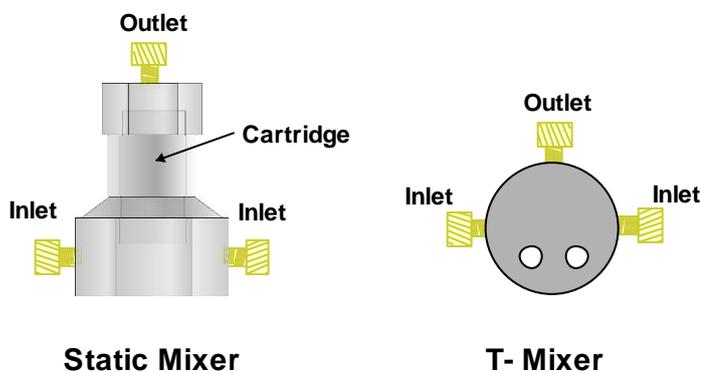
The static mixer consists of 3 parts:
