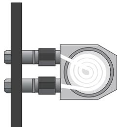
The measuring cells are designed as modules and are therefore easy to replace. They are inserted into the instrument from the front and fixed by two screws.
