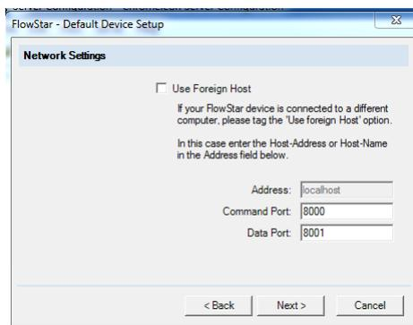
When the FlowStar<sup>2</sup> is connected to the local PC where Chromeleon is running, retain all default values for the address, command port and data port. If "Use Foreign Host" is activated the hostname of the PC must be entered on which the FlowStar<sup>2</sup> controller runs. Port numbers should not be changed. Click on
