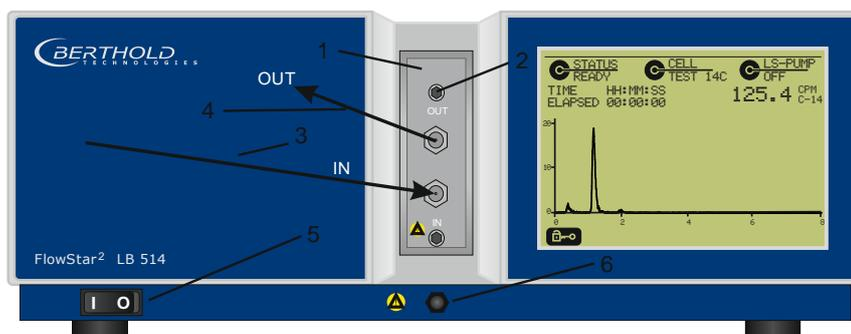
Figure 4: Front view of Radioactivity Monitor
