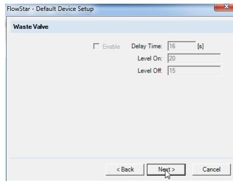
Parameter entry is only possible if the waste valve is activated in the configuration of the FlowStar<sup>2</sup>. After clicking on **Next >** the configuration is finished. By clicking on **Finish** the dialog box will be closed and the FlowStar<sup>2</sup> is configured properly. The Server configuration will look like shown below, depending on the devices used:
