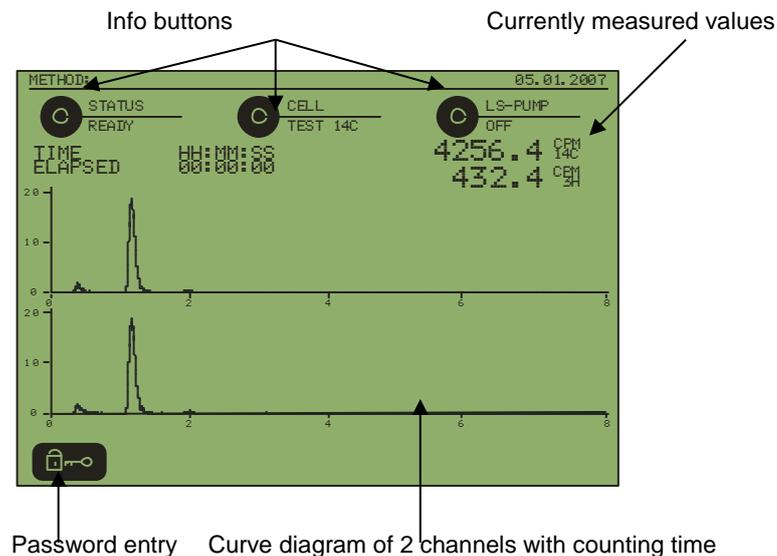
Figure 19: Measurement menu after power on
