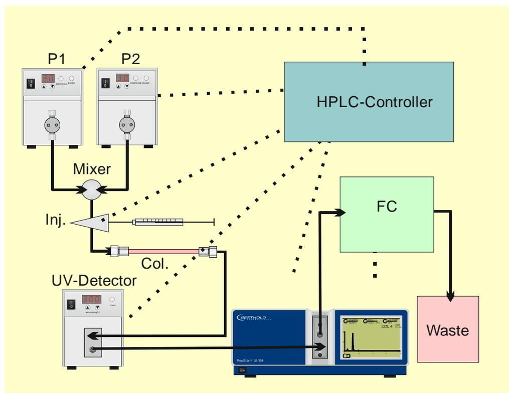
Figure 15: Configuration with solid cell
