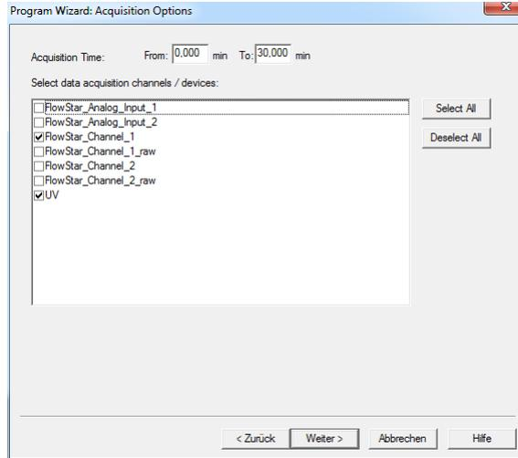
All required signals must be checked. The channels labelled with “.raw”, represents raw data channels without any calculated corrections.
