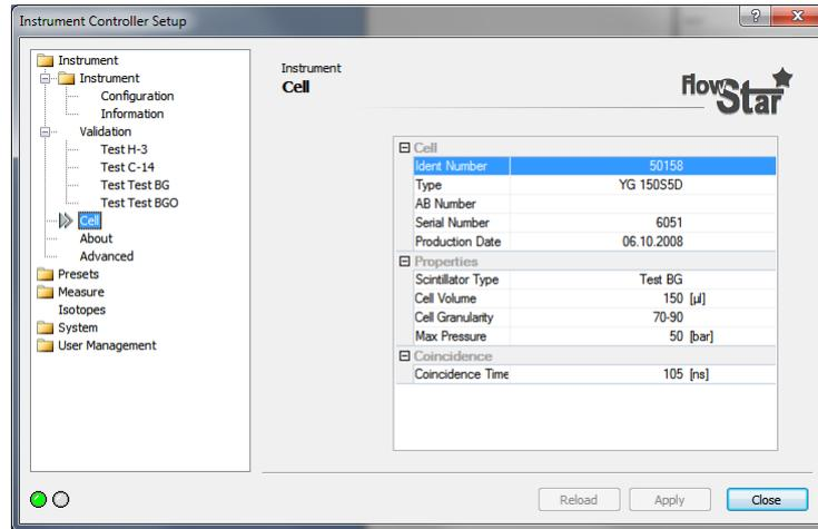
Cell information is available in the “Cell” tab. All information such as ID number, serial number, production date, cell type, volume etc. which are stored on the chip in each individual cell are displayed in this window.
