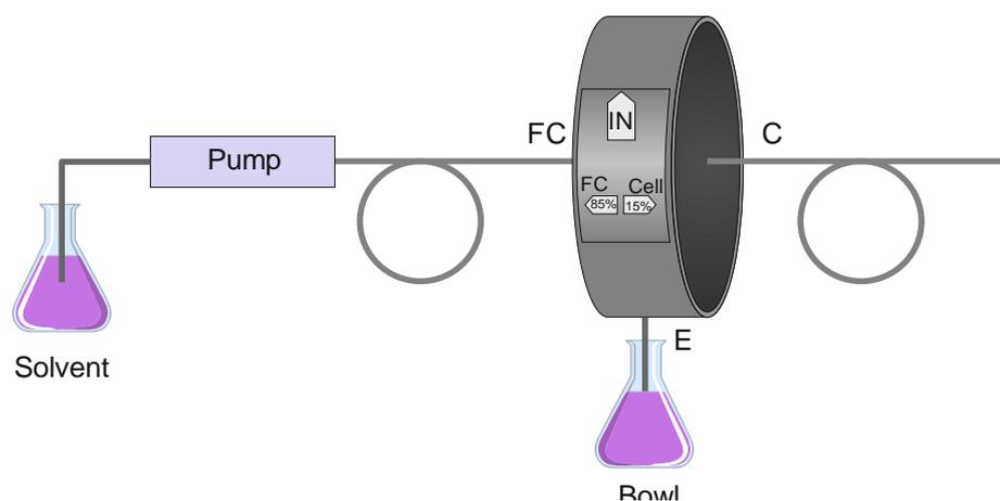
Figure 14: Cleaning capillary or separator
