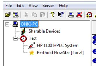
**The possible different configurations (measuring cells, flow rates etc.) are saved locally at the PC where the configuration was done. This means a configuration might not be available using specific client Servers setup structures (server and server configuration done on different PCs. In this case the configuration files (\*.XFS) can be copied manually from the source PC (path C:\Program Data\flwctrl\data)**
