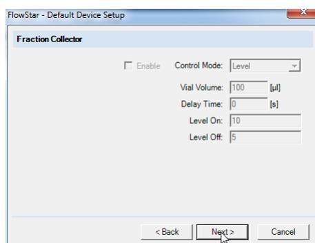
Parameter entry is only possible if the fraction collector is activated in the FlowStar<sup>2</sup> configuration. When clicking on  the waste valve parameters can be entered.
