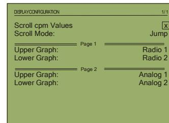
**Jump:** If the measurement curve has reached the right edge of the display, the measurement image jumps to the left by half a display width.
