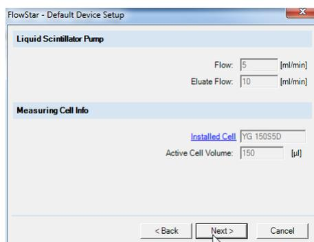
The flow rate for the pump and eluate can be defined in this box. Please note that this function is only available if a liquid scintillator pump is activated in the FlowStar<sup>2</sup> and as well a Z-cell is installed. The flow rate from the eluate is required when cpm, dpm, dps or Bq values should be calculated. By clicking on “installed cell” further information on the currently installed cell will be shown. When clicking on  the fraction collector parameters can be entered.
