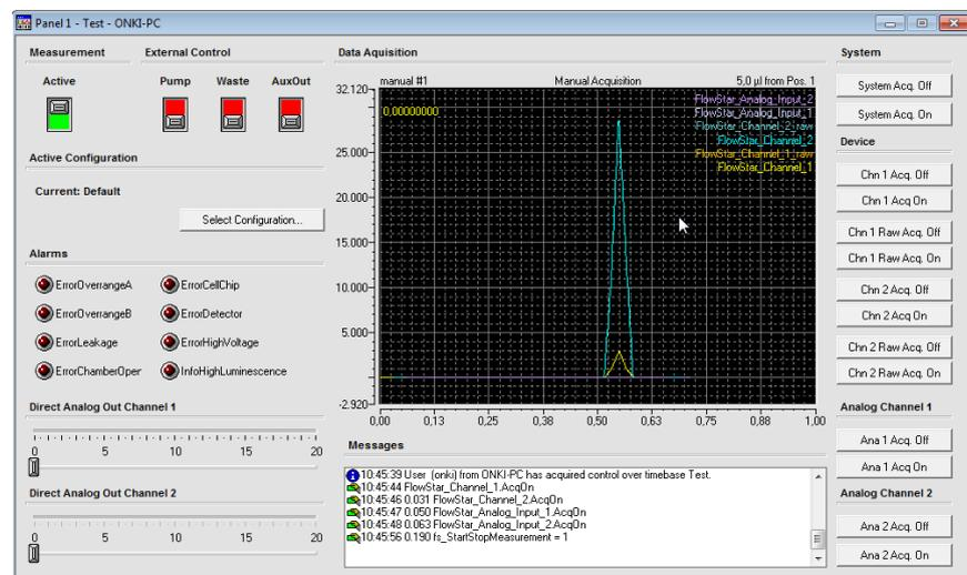
The second panel can display the count rates from the detectors and show the status of the signals. In addition several testing functions are available e.g. to set the analog output voltage to a specific value in order to test the connected A/D converter. Buttons to start / stop the data acquisition are located on the right side of the panel. If no data is shown the Acquisition state must be set to “on” and the measurement mode must be set to “active”
