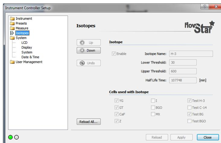
The isotope editor is a tool to browse through the table of nuclides which are stored in the FlowStar<sup>2</sup>. The table of nuclides for the Standard nuclides is read only and cannot be modified. User defined isotopes can be modified. The isotope name, upper and lower threshold for the discriminator and the isotope half life time
