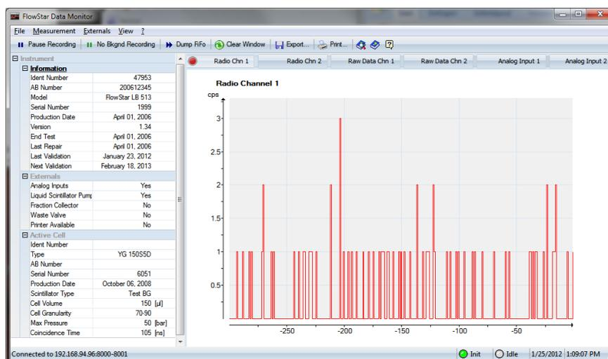
On the left hand side is all relevant information of the instrument available while the current data are shown on the right side. The signal channels are shown in different tabs. By clicking on one of these tabs, the corresponding signal is displayed. On the left side is all relevant information over the instrument such as instrument ID, serial number, firmware version displayed.
