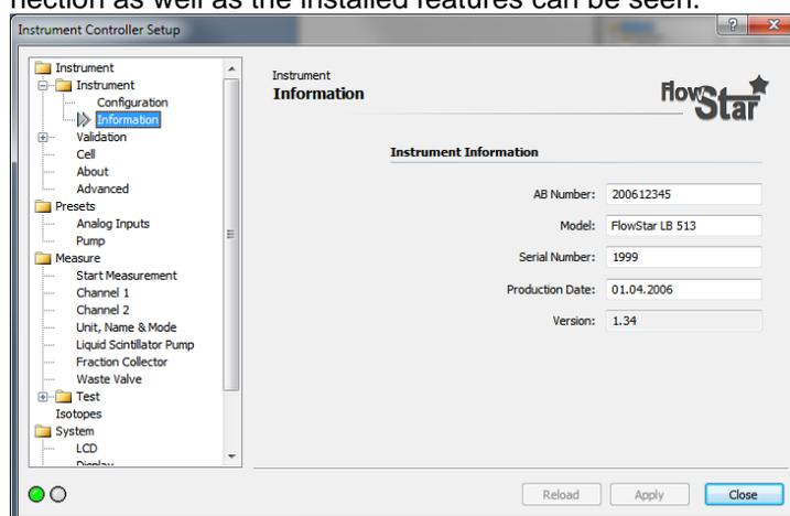
Tab "Instrument information" shows the instrument information such as the order confirmation number of the instrument, model, serial number, production date and installed firmware version number. These information are read only and cannot be overwritten by the controller.
