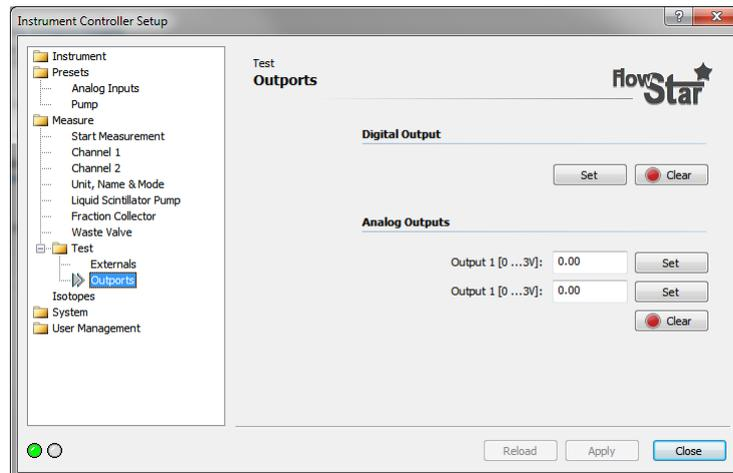
In the Outport section the digital output (AUX) and analog outputs (Ratemeter) can be tested.
