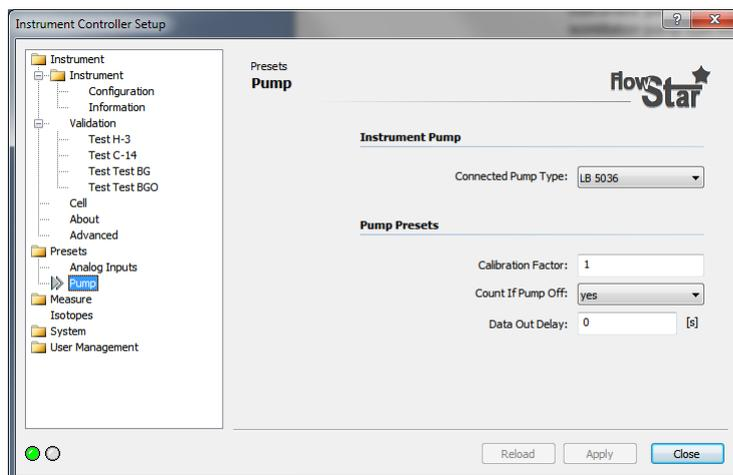
Depending on the pump is used with the FlowStar<sup>2</sup> the correct type must be selected from the list (see chapter 9.1).
