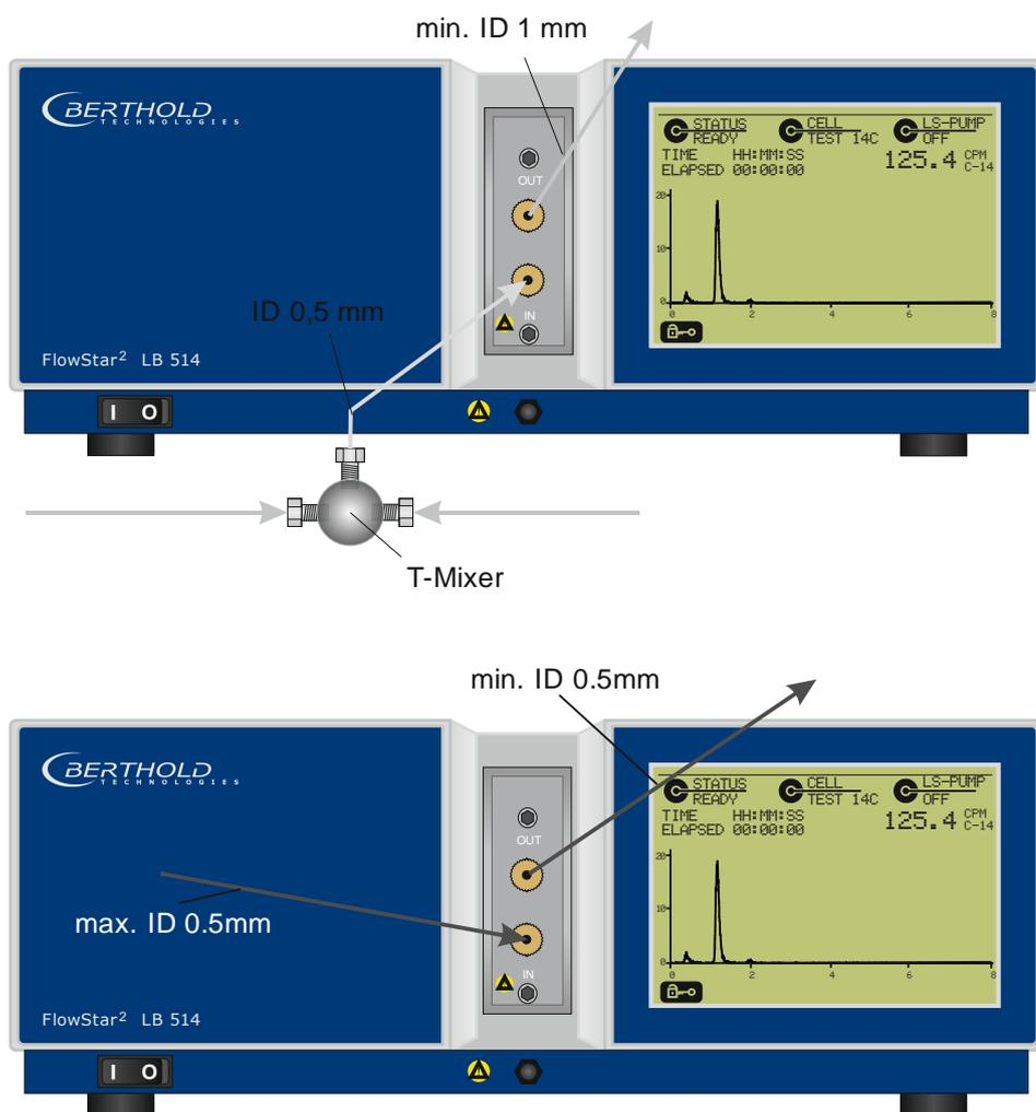
Figure 7: In and outlet capillaries for solid and admixture cells
