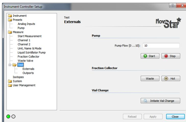
The Test features can be used during setup the instrument or to check if all accessories are properly connected and working.
