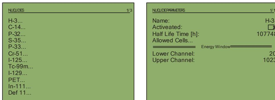
Figure 25: Nuclide table (left); parameters of a selected nuclide (right)
