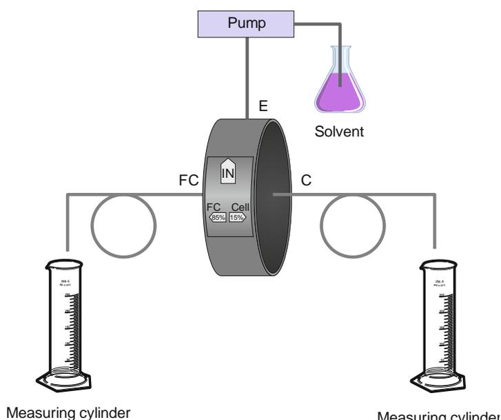
Figure 13: Checking the splitting ratio
