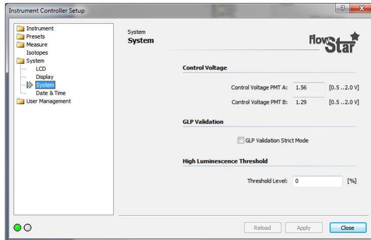
System settings like the PMT control voltage and luminescence warning levels are visible in the “System” tab. PMT control voltages are read only.
