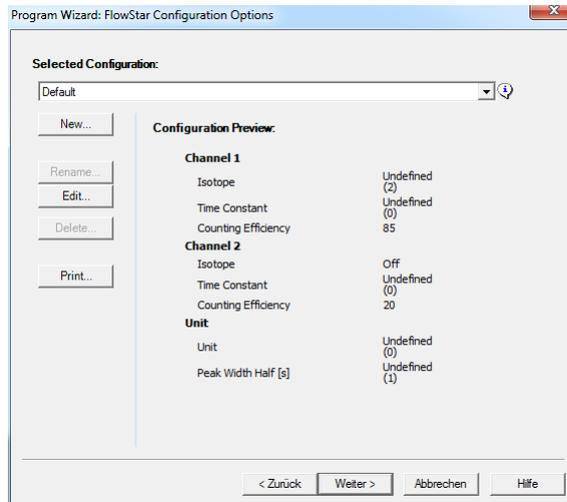
In this dialog the required configuration (Isotope, efficiency, units etc.) can be selected. In case that the required configuration is not available, can be a new configuration created by clicking on **New...**. To modify an existing configuration click on **Edit...**. For print out the selected configuration for documentation purposes click on **Print...**.
