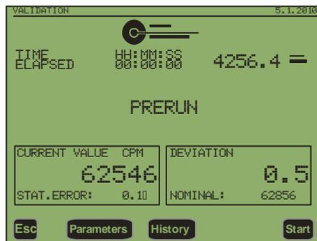
The instrument is in prerun mode. By pressing **<Start>** the validation measurement starts and the current (upper right corner) as well as the integrated value (lower left corner) and the deviation from the nominal value are displayed. If „Prerun“ is still displayed after starting the measurement, a prerun time is defined in the parameters. This prerun time is used to calm down the test cell which could give higher values due to the exposure to daylight.
