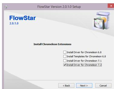
If the FlowStar<sup>2</sup> is connected to the PC and initialized properly, the instrument driver can be installed to the CHROMELEON Server using the “Server Configurator” Tool (Instrument Configuration Manager in CM 7.x). It will look like this:
