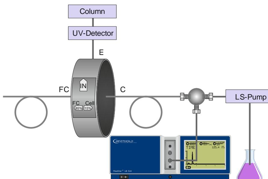
Figure 11: Configuration with Analytic Splitter
