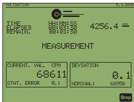
Once the measurement is finished either „PASSED“ or „FAILED“ is displayed, depending if the results are within or outside the specified tolerance level.
