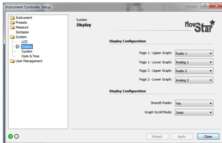
To get 2 pages with full screen signal select any signal in the “upper graph” box and “none” in the “lower graph” box. For further information on these parameters please refer to chapter 9.1.
