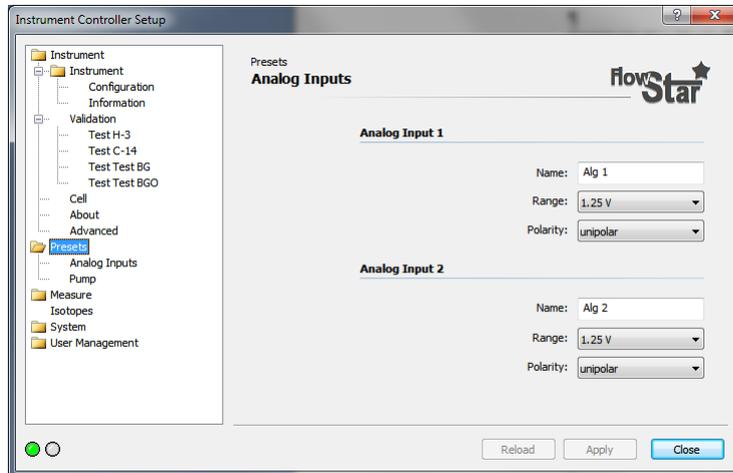
The label of the signal, the voltage range and polarity can be defined for each individual channel (see chapter 9.1).
