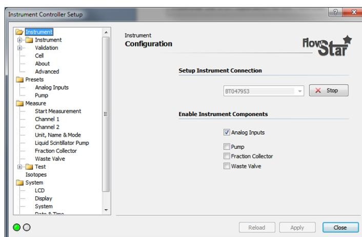
In the tab "Instrument Configuration" the current hardware connection as well as the installed features can be seen.
