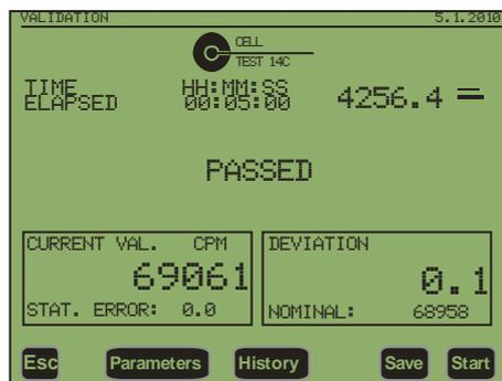
In case of „FAILED“ the measurement can be repeated by pressing **<Start>**. If the validation is „Passed“ the results can be saved pressing the **<Save>** button. A failed validation cannot be saved.
