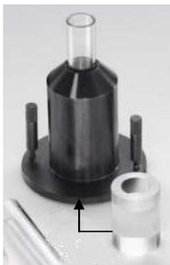
The standard sample holder and the microfuge tube sample holder are suitable for use with injectors. The standard sample holder can accommodate 12mm tubes with a length of 75 and 55 mm. For the 55mm tubes, the Plexiglas insert (included with the shipment) has to be inserted from below. The microfuge tube sample holder accommodates 1.5ml and 2ml microfuge tubes with caps.
