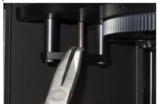
Turn the shaft until the focus drive moved down approx. 5 mm.
