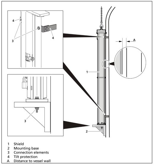
Fig. 6 Installation on vessels
