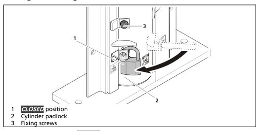
Fig. 10 Shield closed (*CLOSED* position)
