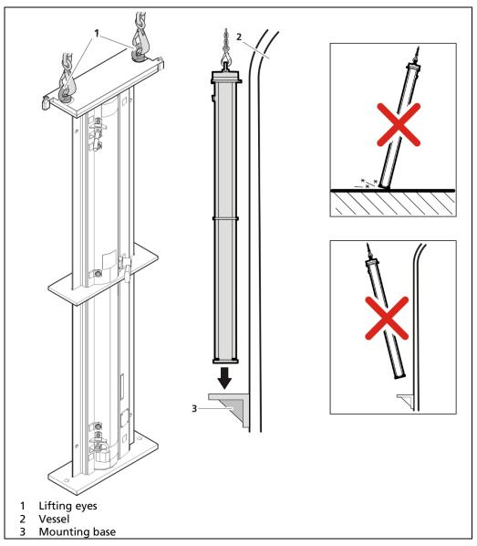
Fig. 5 lift and lower the shield
