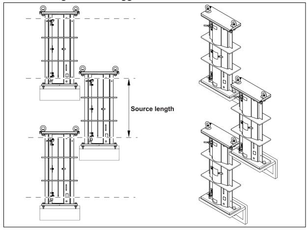
TI-Abb. 6 Mounting variants staggered (example illustration)
