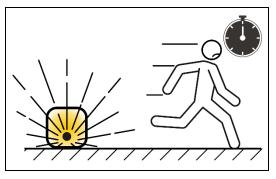
Any work required in the vicinity of radiometric measuring systems is to be prepared for carefully and to be organised in a way that the work can be executed as quickly as possible. Here, providing the correct tools and aids is particularly important.
