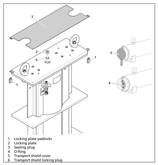
Fig. 14 Prepare the installation
