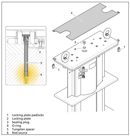
Fig. 12 Make the source accessible
