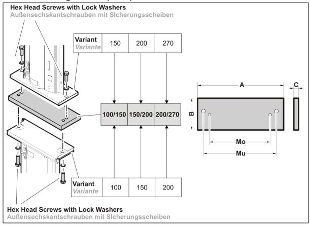
TI-Abb. 4 Mounting Kit Adapter Plate
