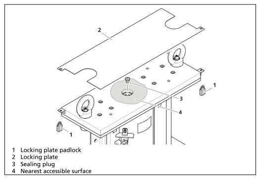
Fig. 11 Nearest accessible surface for leak test
