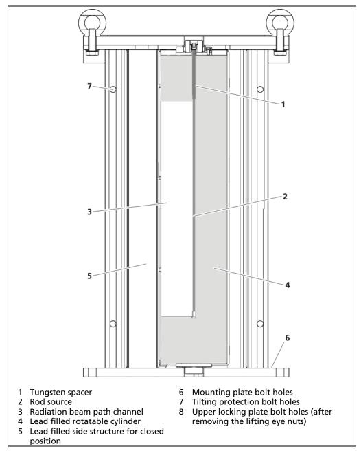
Fig. 3 Sectional view (position CLOSE)
