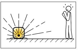
If work close to equipment containing radioactive substances is required, the largest distance possible is to be kept. In particular, this applies to employees not immediately required to work directly with the radioactive devices.
