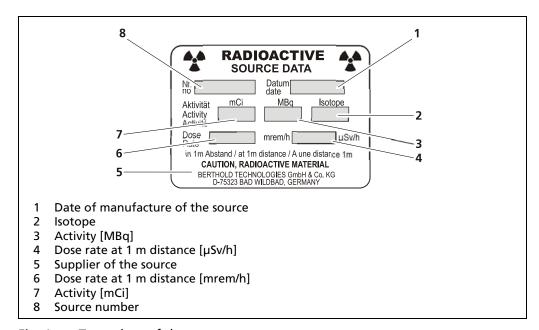
Fig. 1 Type plate of the source
