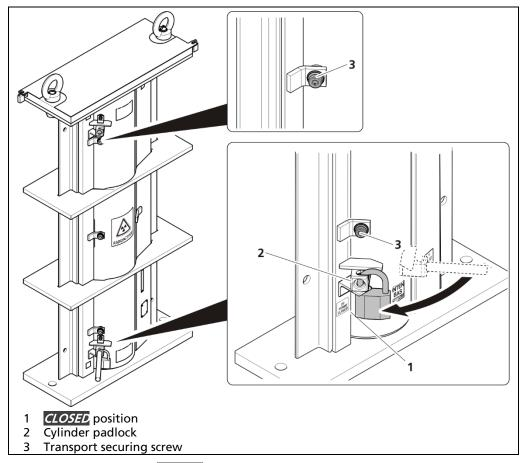
Fig. 4 Shield closed (*CLOSED* position)
