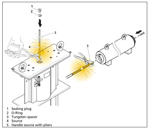
Fig. 15 Installing the source in the shield
