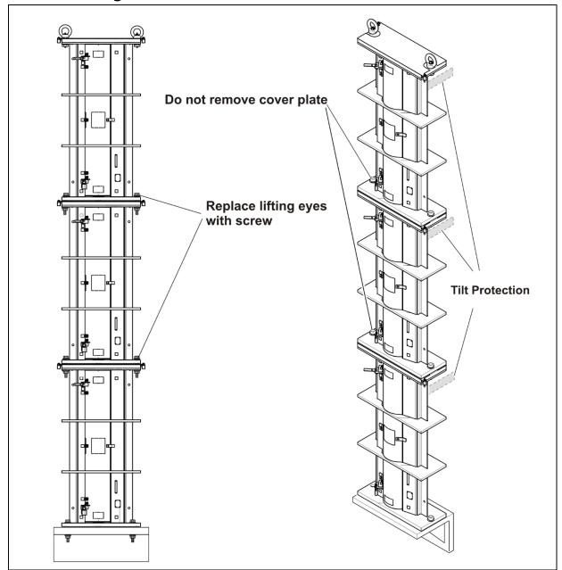
TI-Abb. 5 Mounting variant stacked (example illustration))
