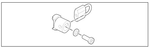
Fig. 9 Locking tool set (Mat. No. 73883)
