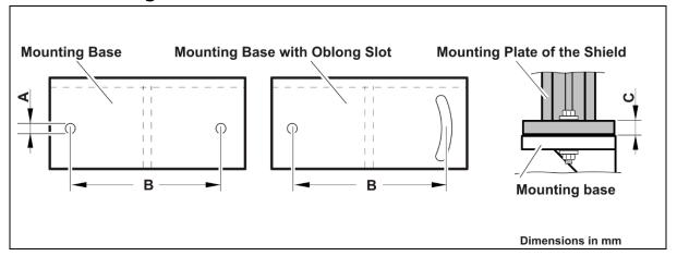
TI-Abb. 3 Mounting base dimensions for LB 8300 Rod Source Shields
