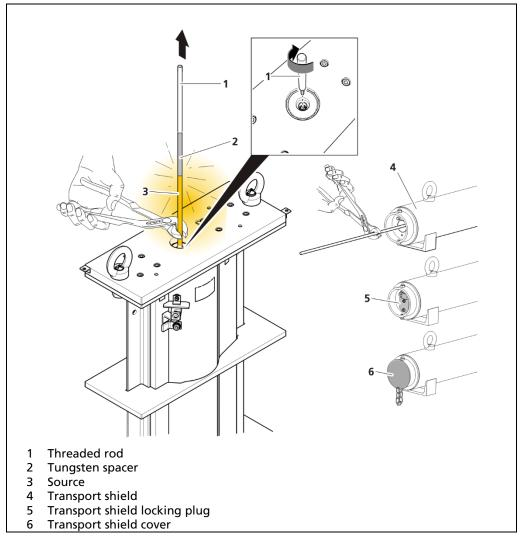
Fig. 13 Remove source out of shield
