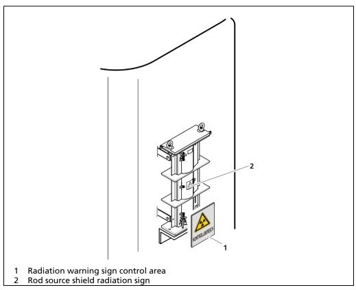
Fig. 7 Example marking
