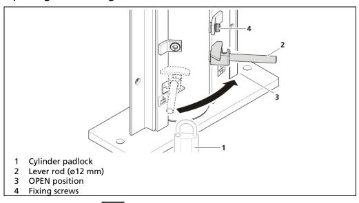
Fig. 8 Shield open (*OPEN* position)
