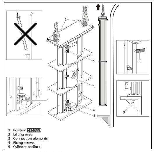
Fig. 16 Dissasemble the shield
