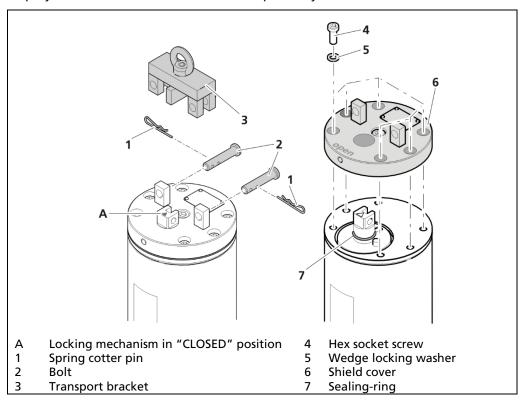
Fig. 15 Inspection and replacement of the sealing ring
