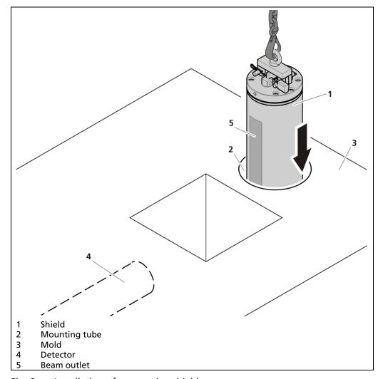
Fig. 6 Installation of a operation shield
