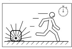
Any work required in the vicinity of radiometric measuring systems is to be prepared carefully and to be organised in a way that the work can be executed as quickly as possible. Here, providing the correct tools and aids is particularly important.
