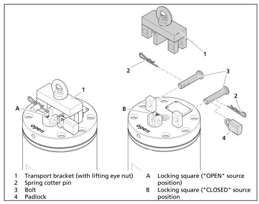
Fig. 5 Operation shield with transport bracket and source. Position left: "CLOSED", right: "OPEN"
