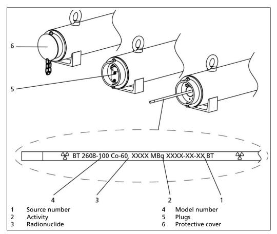
Fig. 9 Usage of a transport shield
