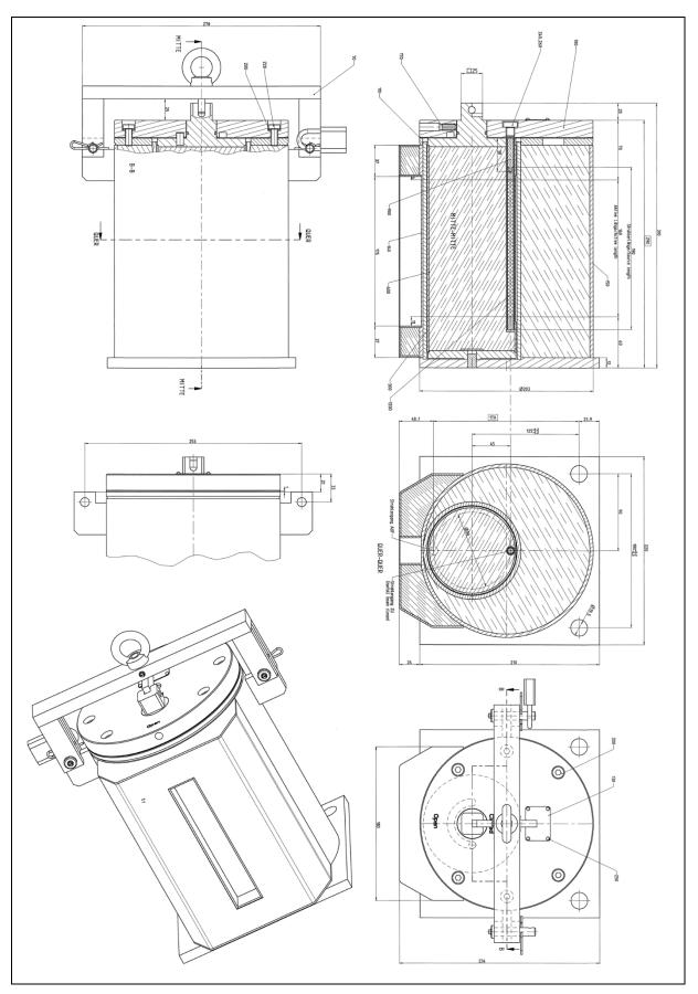
Fig. 20 Example Drawing Mold Level Shield with Collimator
