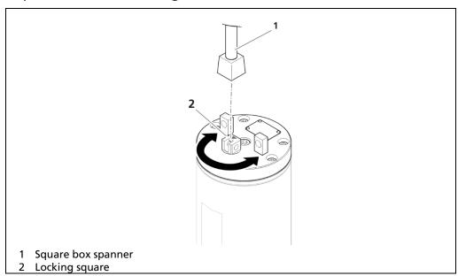
Fig. 13 Open and close the locking mechanism
