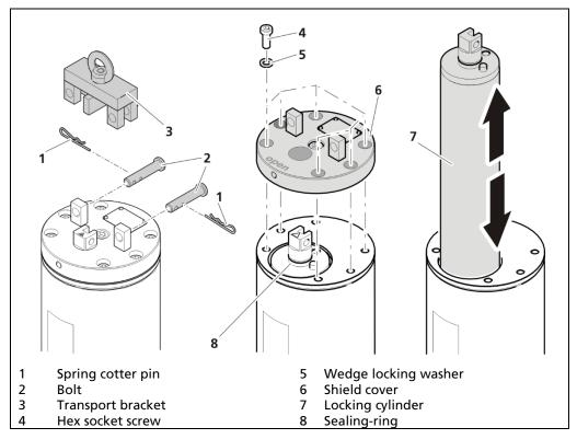
Fig. 14 Dismounting and mounting the locking cylinder of a operation shield
