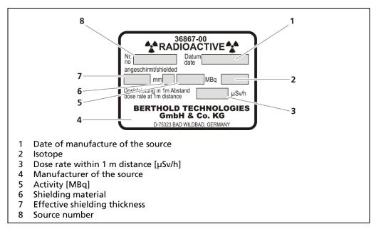
Fig. 1 Type plate of the sources
