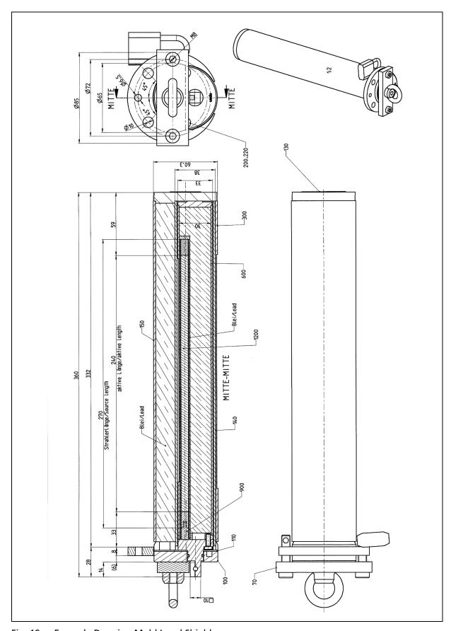
Fig. 19 Example Drawing Mold Level Shield
