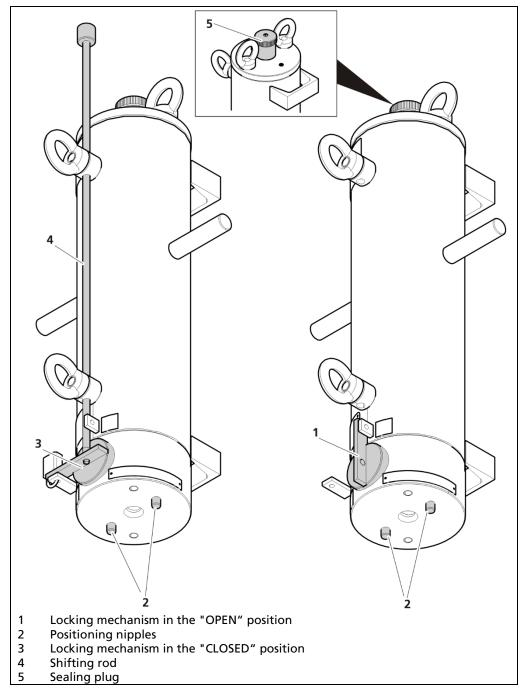
Fig. 7 Left: Locking mechanism in the "CLOSED" position, secured by shifting rod, right: Locking mechanism in the "OPEN" position
