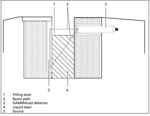
Fig. 12 Source without operation shielding within the water Box of the mold
