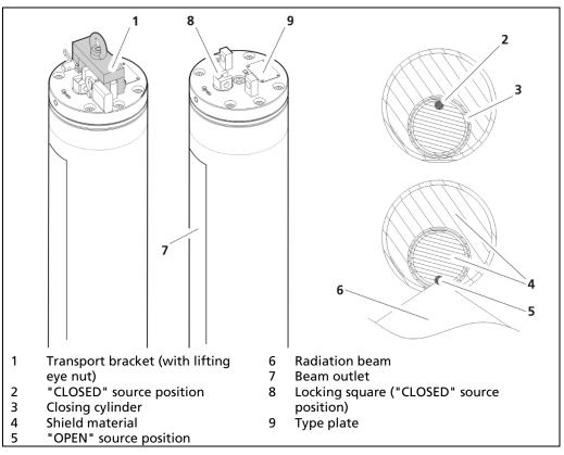
Fig. 2 Basic structure of operation shield
