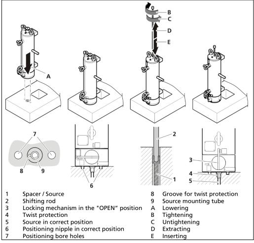
Fig. 8 Mounting the source
