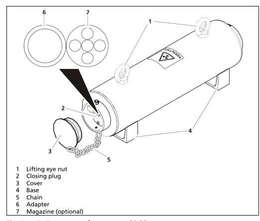
Fig. 4 Basic structure of a transport shield
