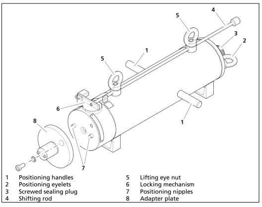
Fig. 3 Structure of a transfer shield
