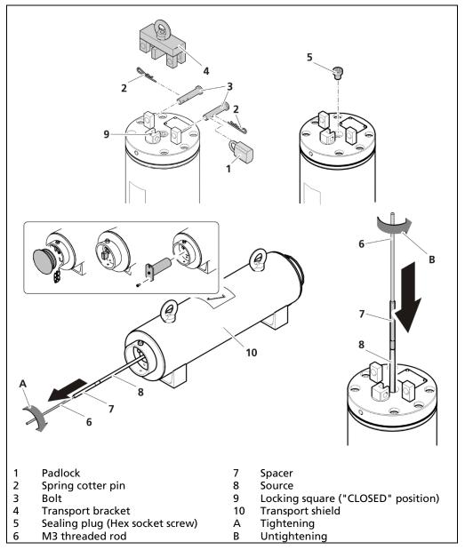
Fig. 17 Installation of the source into a operation shield
