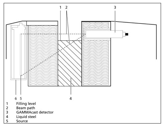
Fig. 11 Outside of the water box of the mold
