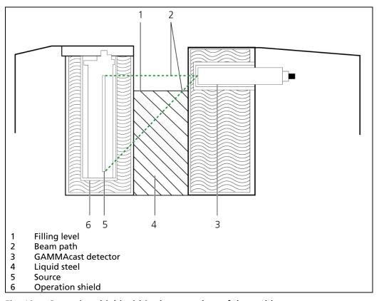
Fig. 10 Operation shield within the water box of the mold
