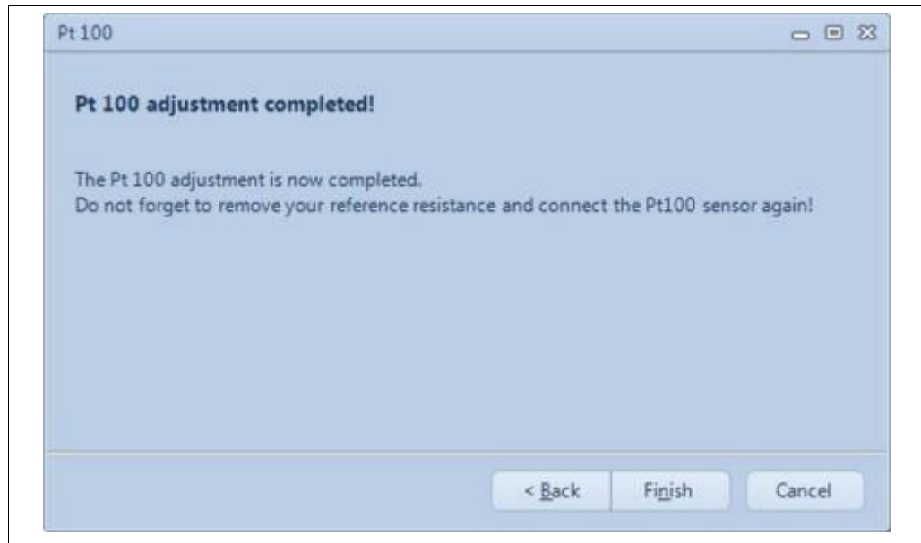
Fig. 45 Last Step of the Pt100 Wizard
