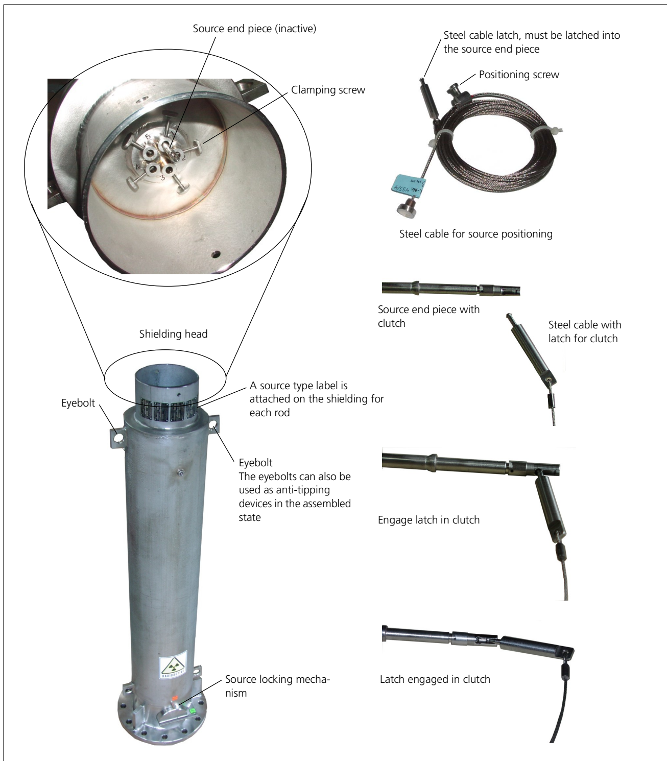
Fig. 2-32 Flange shielding with steel cable
