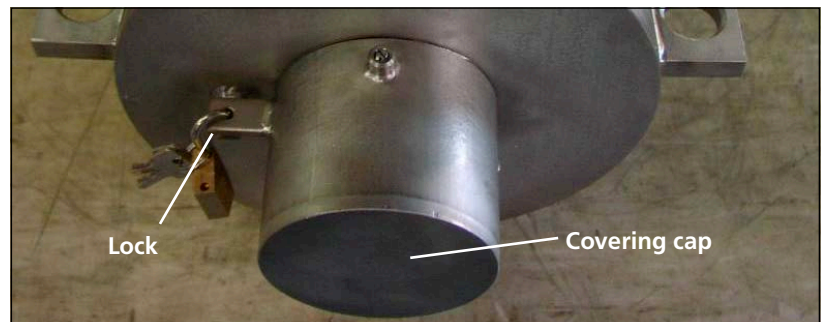
Fig. 2-33 Lock and covering cap
