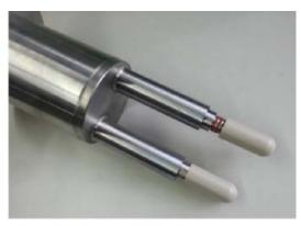
Figure 5-1: Replacing the plastic caps of the measuring rods
