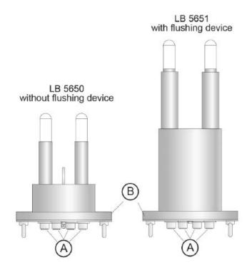
Figure 3-11: Container probe versions
