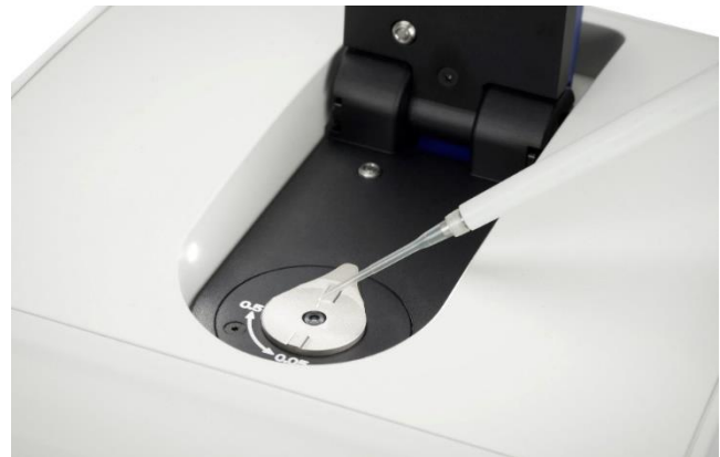
Figure 4: pipetting in the sample area of the Colibri+
